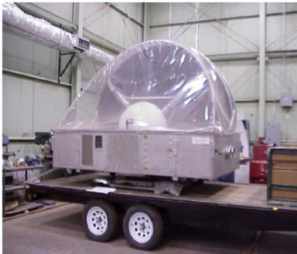
Figure 2-9. High intensity JOLT hyperband generator used in the United States.
