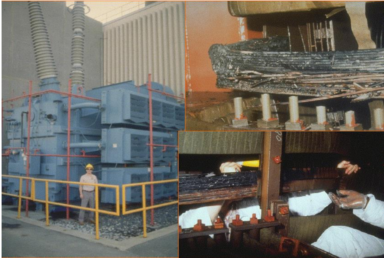
Figure 2-33. Damaged transformer at the Salem Nuclear Plant.
